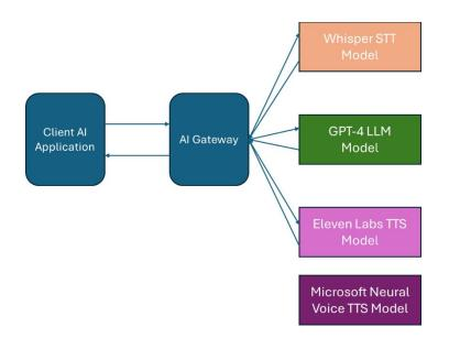
When using an AI Gateway, the client application is no longer directly connected to AI resources. In fact, it only requires a single connection to the AI Gateway. The client application may be coded and deployed independently from the model infrastructure. In addition, changes to AI resource can be automatically handled by the AI Gateway, which simply re-routes incoming calls to the alternate resource, while the client application remains unaffected.
