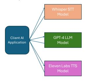
As you can see, the Client AI Application must manage communication with each AI resource independently. And if one of the resources changes, for example, if Microsoft Neural Voice is substituted for Eleven Labs, then the Client AI Application must be updated and redeployed.
